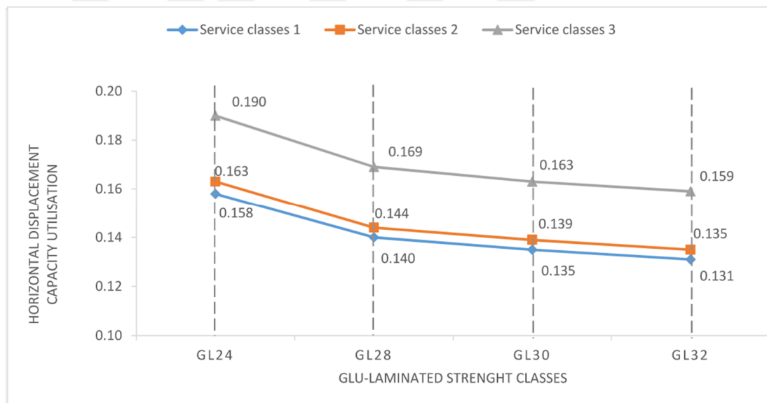
Figure 4.33 : Portal Frame Horizontal Displacement SLS Capacity Utilisation.
