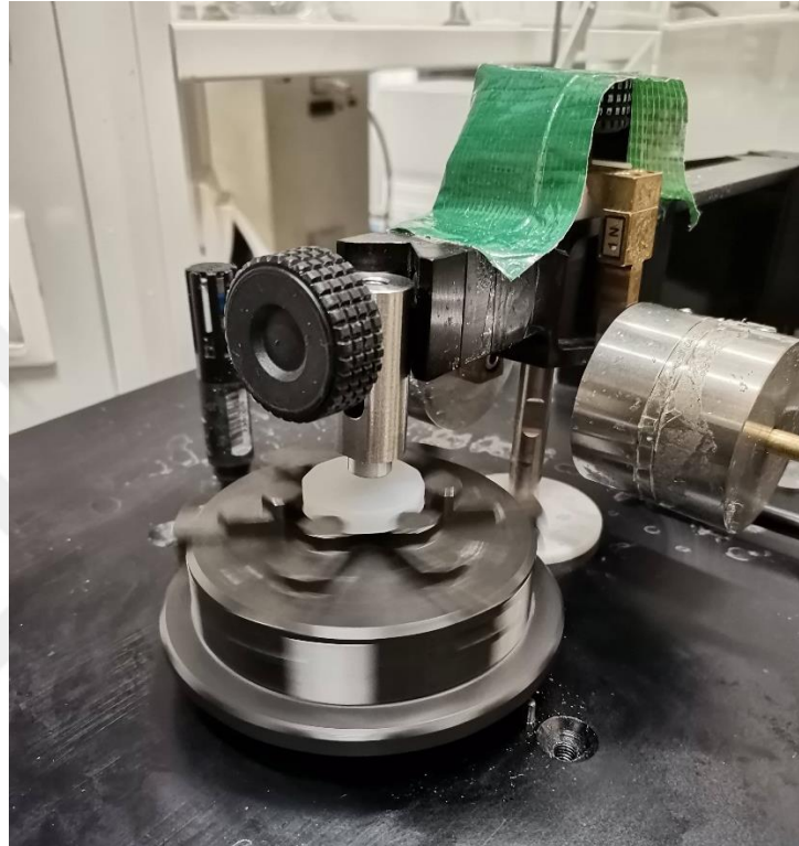
Figure 5.6 Ball-on-disk testing setup.
