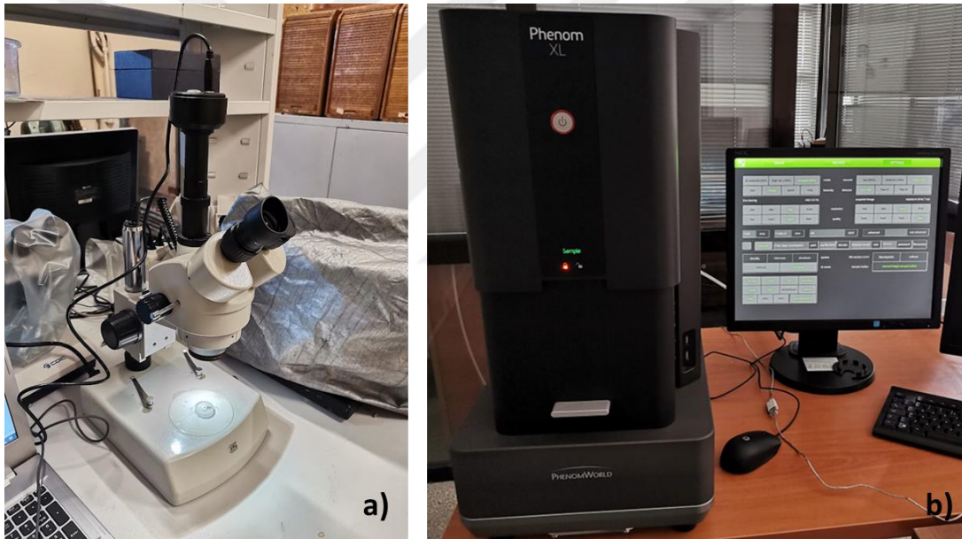
Figure 5.7 Imaging instruments: a) light microscope, b) SEM.
