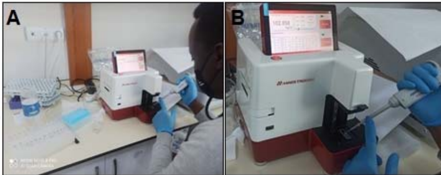
Figure 3.5. Spectrophotometer during DNA samples analysis. (A) broad and (B) close-up photos
