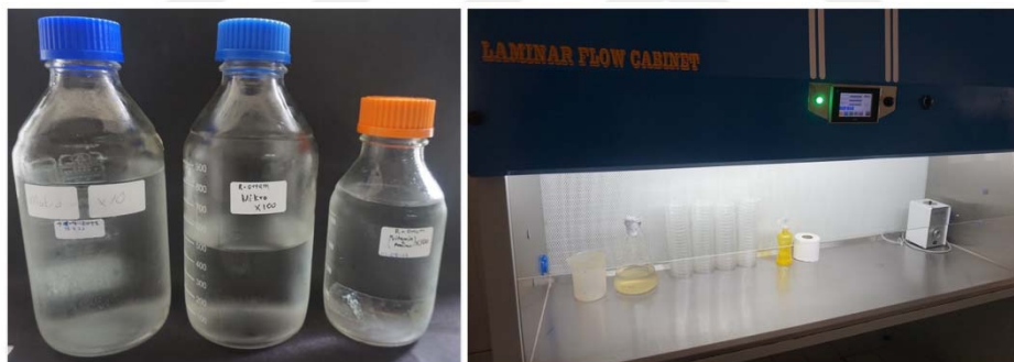
Figure 3.17. Nutrient media preparation (A) Three type of stock solutions used during media preparation, (B) Prepared medium and petri dishes in the bench just before dispensing the medium
