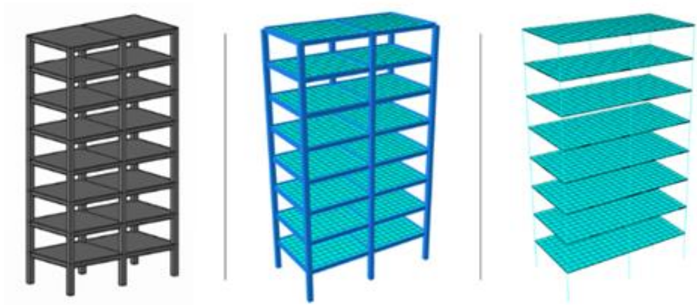
Figure 10: The eight-story building (a) CAD model (b) Finite element meshed parts
