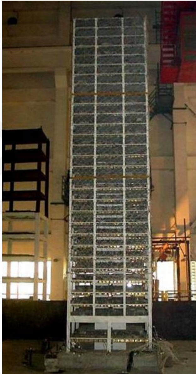
Figure 2.3: The scaled model produced for shake table test in laboratory environment [49].
