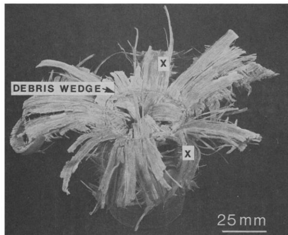
Figure 1.18. Crush zone of a [0/90/90/0] glass fibre-polyester resin tube [10].
