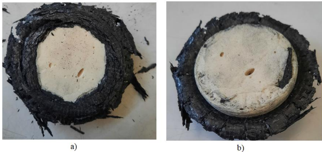
Figure 4.16. Crushing mode of PU foam filled tube, a) with debris wedge, b) debris wedge removed.
