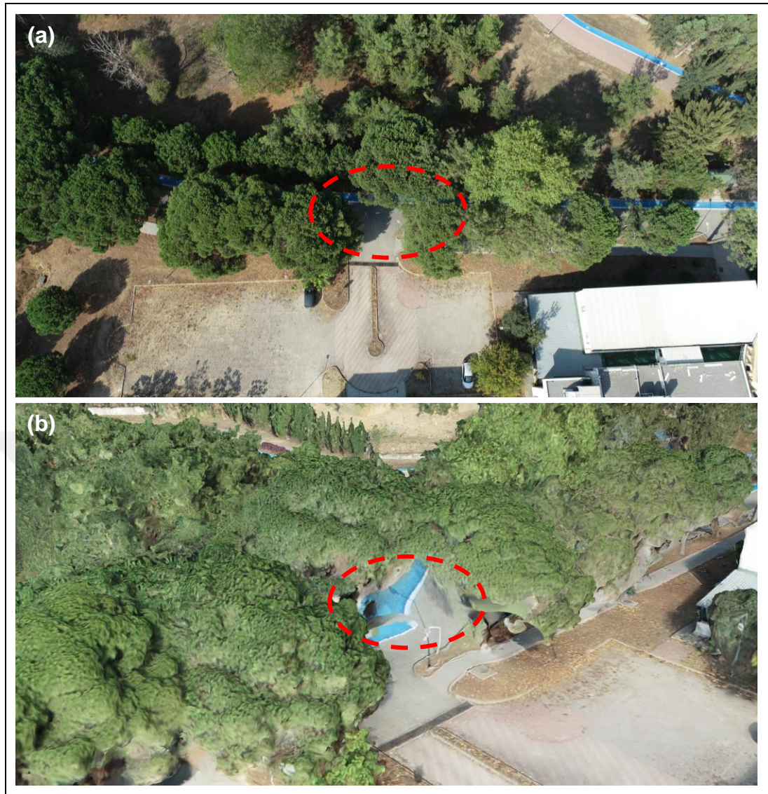
Figure 6.2: a) An aerial photo of the GTU Campus. b) The 3D textured mesh model of the region covered by dense trees.
