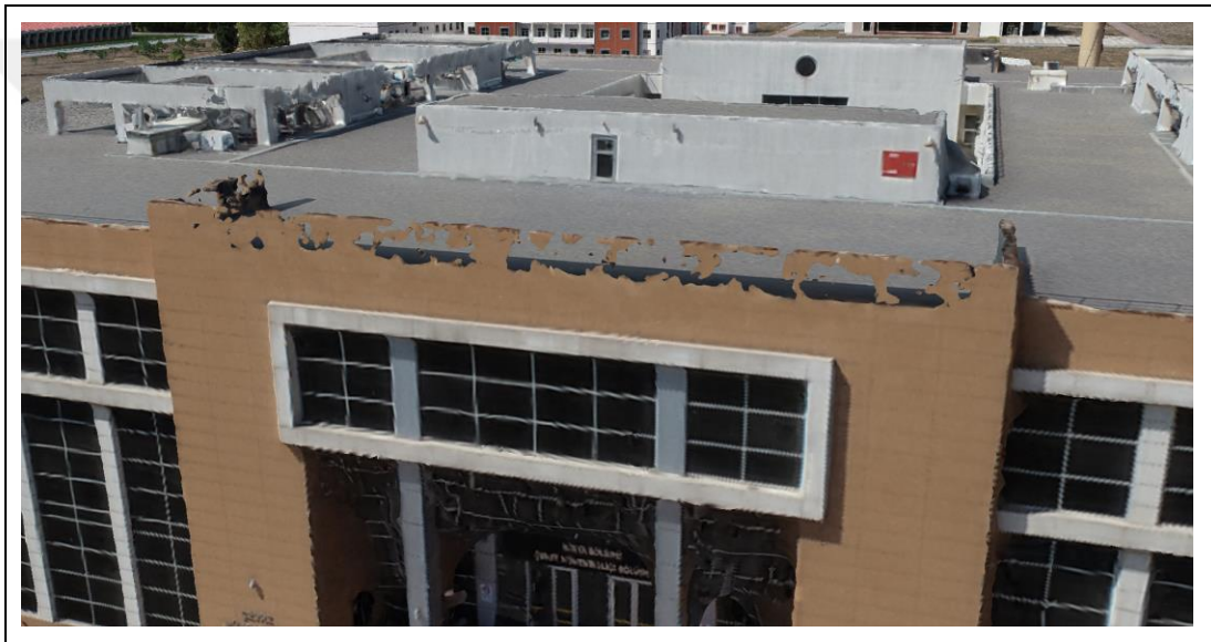
Figure 6.1: Interpolation effect on a rooftop wall due to points with low correlation.
