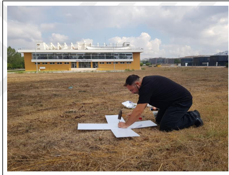
Figure 4.4: The establishment of a GCP.
