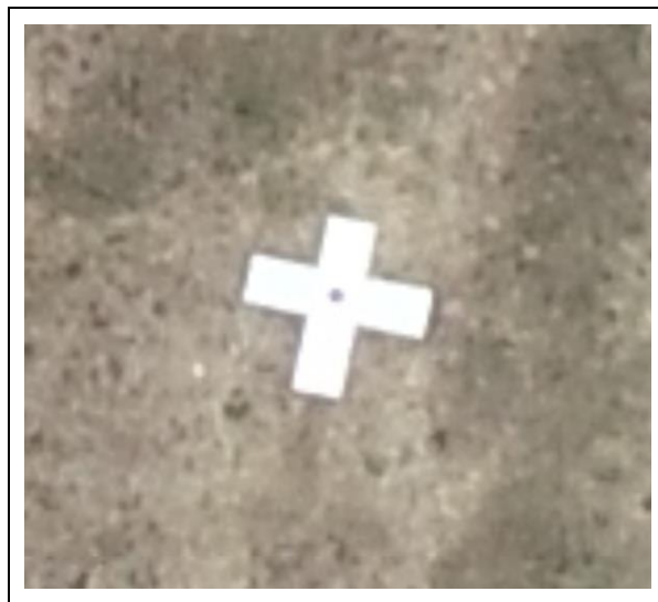
Figure 3.4: A polycarbonate GCP consisting of two combined sheets.
