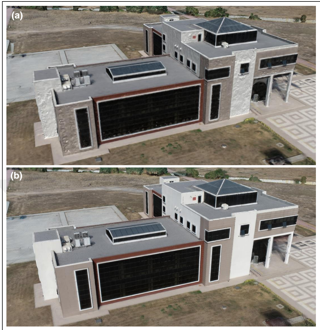
Figure 4.14: a) A 3D mesh model without texture. b) A 3D mesh model with texture.
