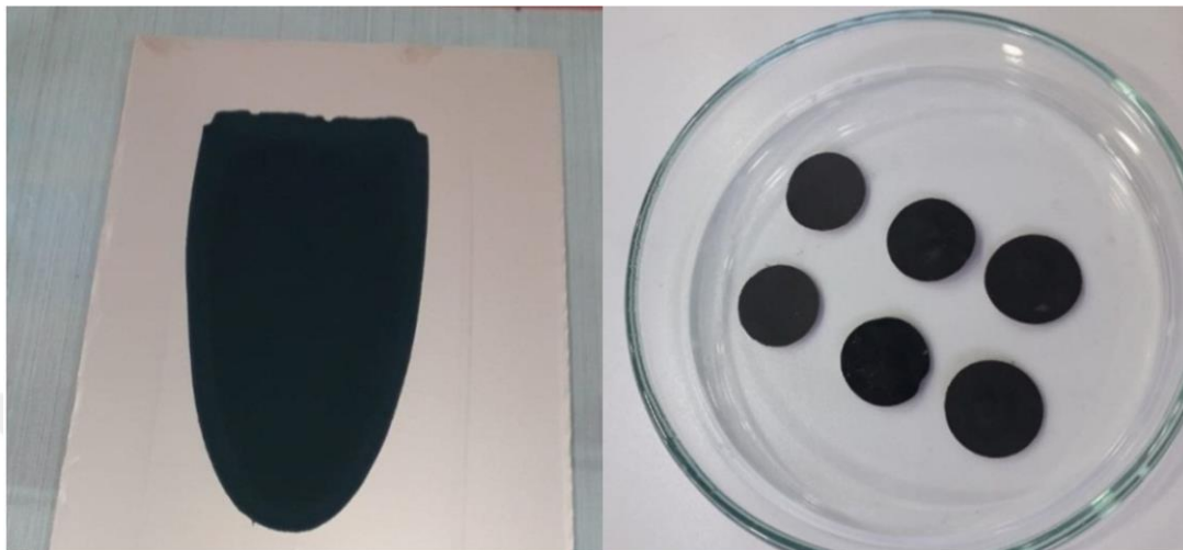
Figure 3.3. Pasted slurry on a copper foil and electrode discs
