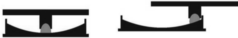
(a) Single Pendulum bearing cross section
