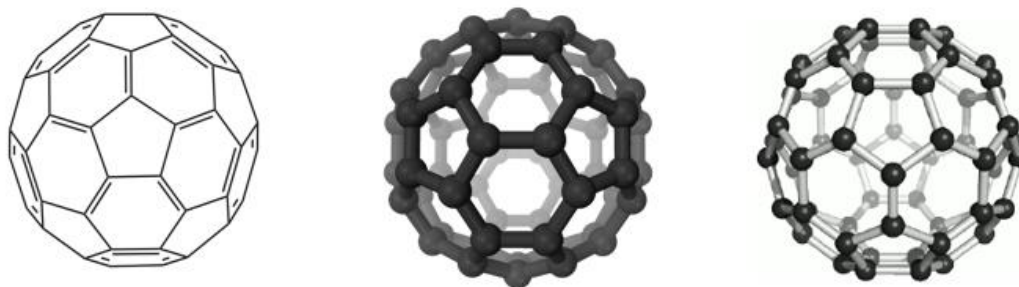
Figure 2.3 : Three different illustration of buckminsterfullerene, C_{60} .
