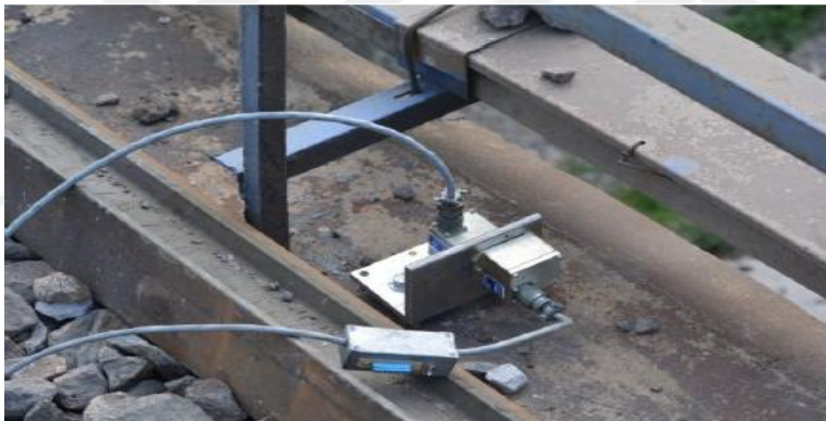
Figure 4.10 : An example bi-axial accelerometer unit.
