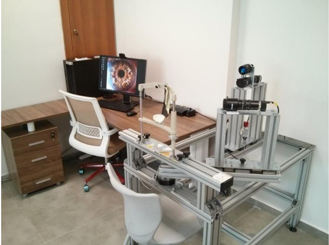
Figure 0.1. Experimental setup of Melikşah University off-angle iris dataset.
