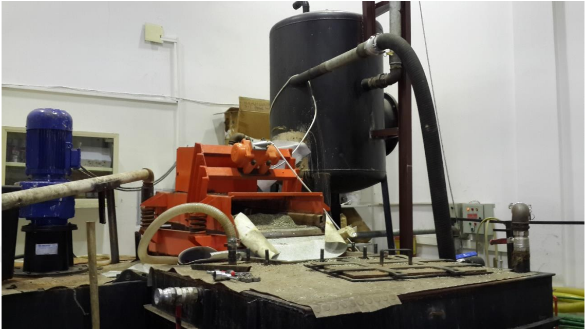
Figure 19. Solid Separation System and Cuttings Collection Tank
