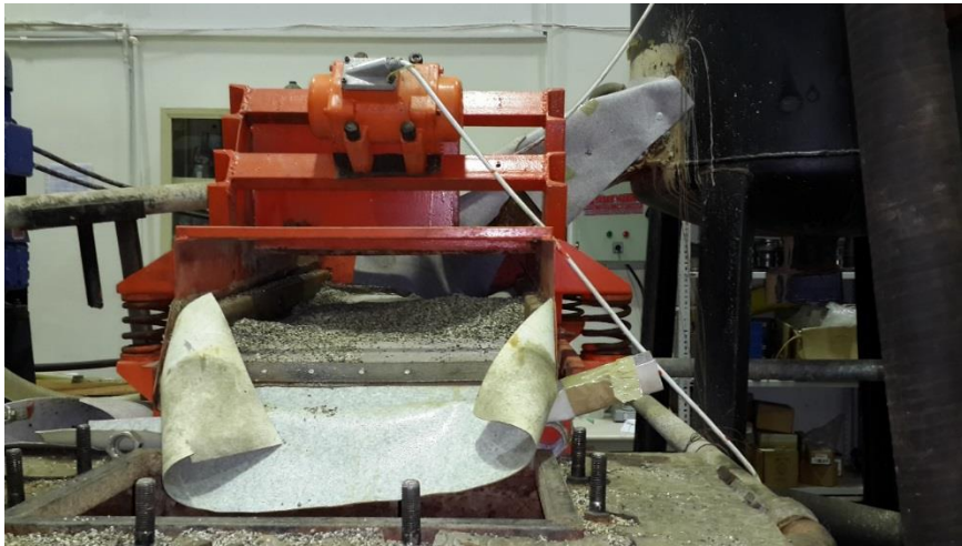
Figure 18. Solid Separation System - Shale Shaker
