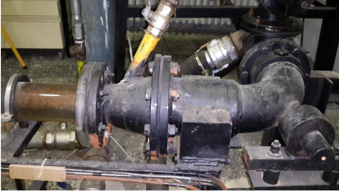
Figure 14. Gas Liquid and Cuttings Inlet to the Flow Loop Test Section – 1
