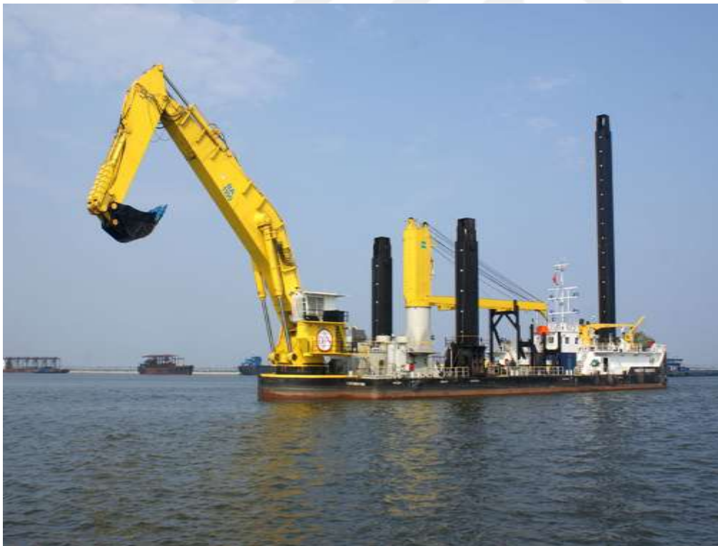
Figure 3.9 : The backhoe dredger ( http://www.jandenul.com ).
