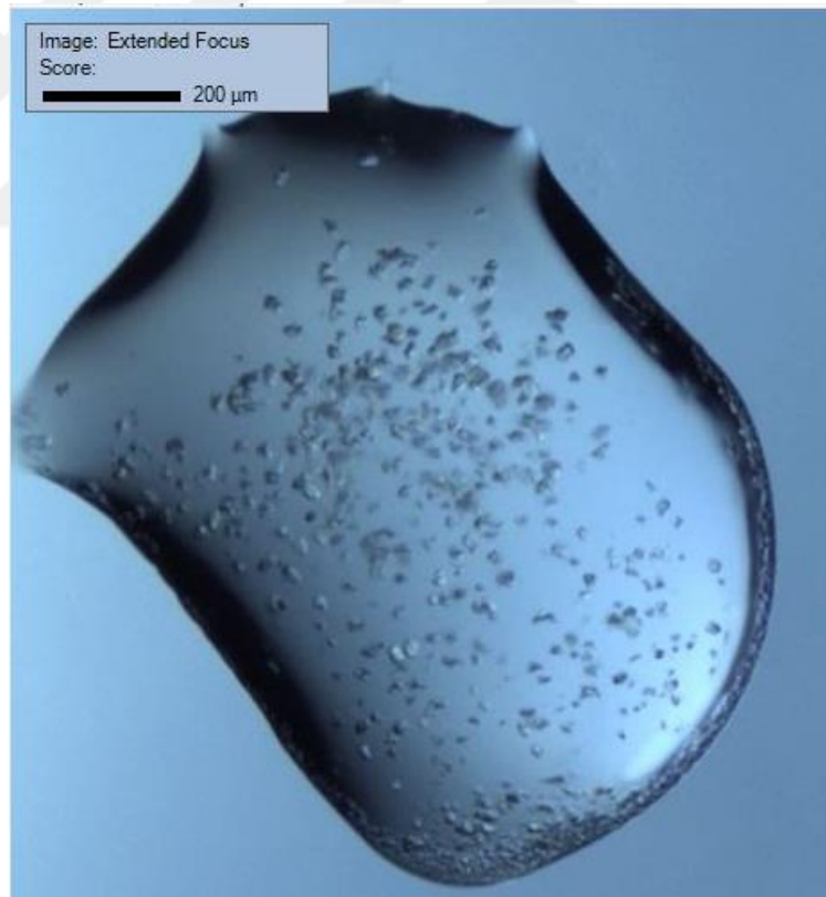
Figure 3.11: ANK E1929-G2126 protein crystals from initial screenings with/without compound I (Table 2.2) with 1% DMSO added buffer conditions. A: Crystal formation with ANK E1929-G2126 in 0.1M MES, 20% PEG6K and 1% DMSO. B: Crystals of ANK E1929-G2126 with compound I with 0.2M Sodium Sulphate, 20% PEG3350.
