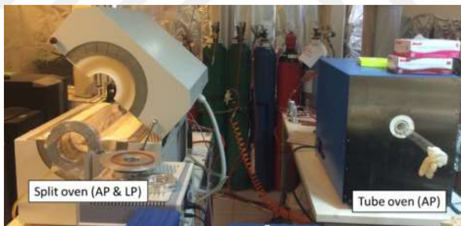
Figure.3.1 : Split oven (left) and tube oven (right) setups which have been used for CVD grown graphene production [51].
