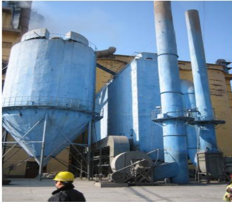
Figure 4.6. Cyclone and filter for cleaning exit gasses in VSKs (Viacrozc,2005).
