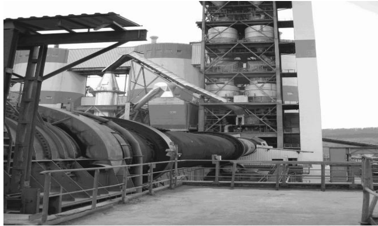
Figure 5.7. Cement kiln equipped with cyclone pre-heaters (SCI,1998).
