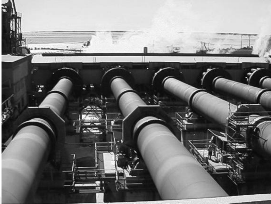
Figure 5.6. Wet, long cement kiln (SCI,1998).
