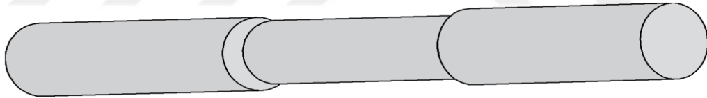
Figure 5.4. Schematic diagram of dumbbell-type rotary kiln (SCI,1998).
