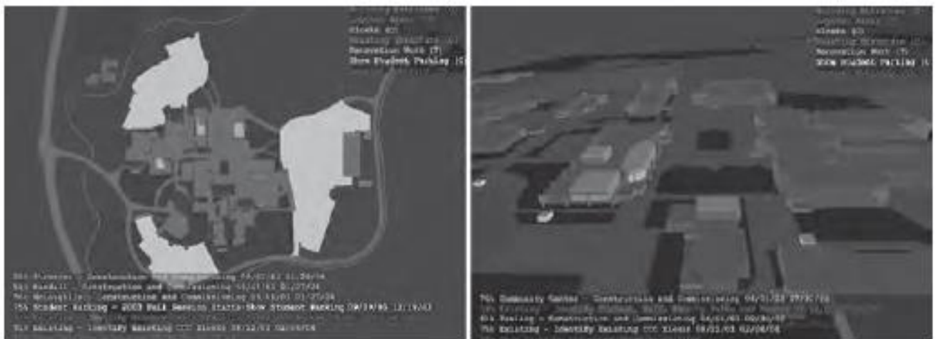
Figure 4.7 "4D snapshots of a campus wide project showing various construction activities occurring throughout the campus to landscape, road, and facilities"(Eastman, 2008)
