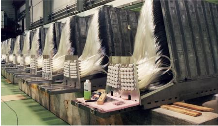
Şekil 3.8. Hadronik İleri kalorimetre (HF)' in kamaları ( http://www.fnal.gov/pub/today/images/images04/Calorimeter_Wedges.jpg )
