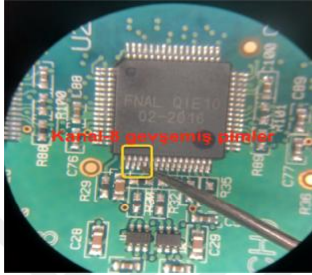
Şekil 4.7. (e) Kanal 8 gevşemiş pimler (Problems with card 634, Noonan, D., 2016) https://indico.cern.ch/event/563683/contributions/2277974/attachments/1324599/1988156/ProblemsWithReworkQuality.pdf
