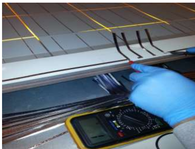
Figure 4.2.6 Short Circuit Test
