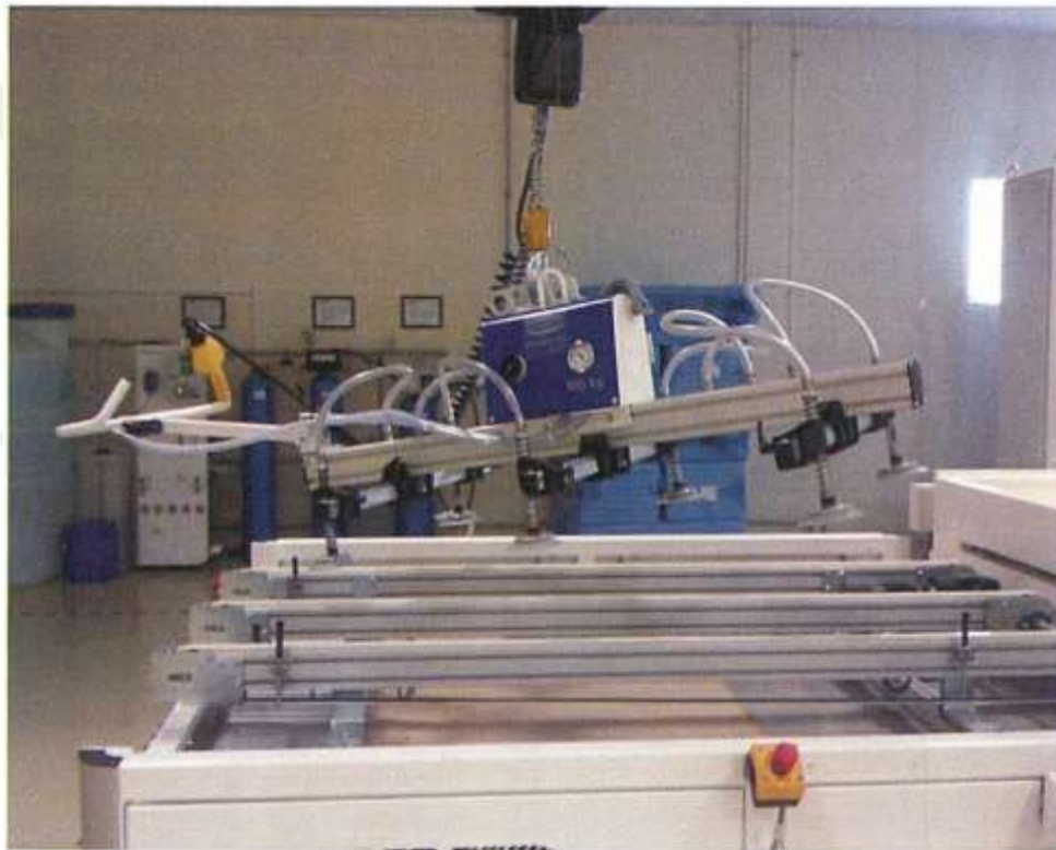
Figure 4.1.2 Glass Loading Machine [12]
