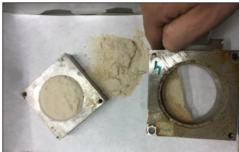
Figure 3.7. The crust formation at the top half of the direct shear box
