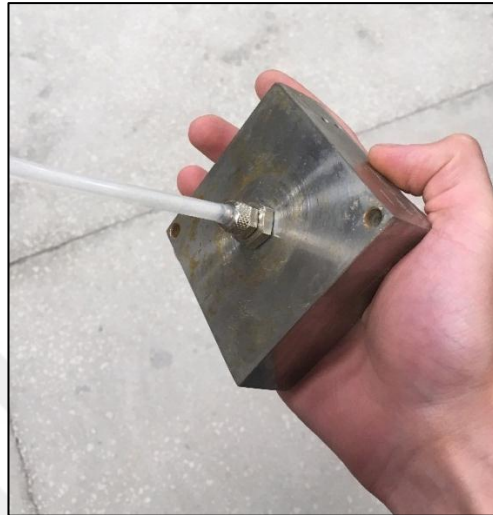
Figure 3.10. Silicone hose connection to the direct shear test box
