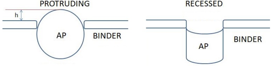
Figure 3.3: AP Particles Protruding and Recessing at Surface.
