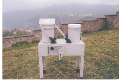
Figure 4.2 Automatic rain collecting system (İlhan et al., 2006)
