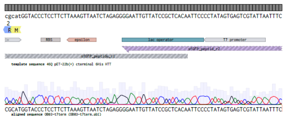
Figure D.21 1: The result indicating the sequence analysis of the peptide against Htt-46Q fused with sfGFP.
