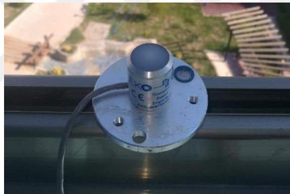
Figure 4-4. Pyranometer Used in Data Collection Points
