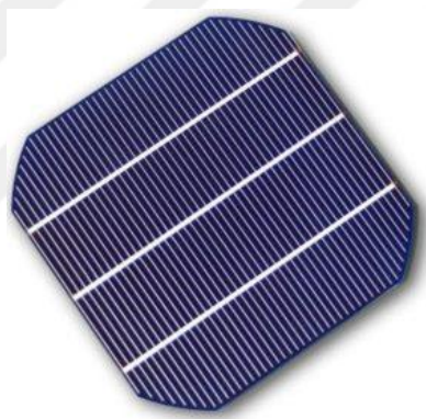
Figure 2-7. Single PV Cell [33]
