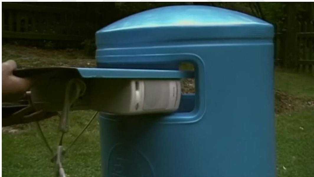
Figure 4.23: Installation of the sound players, speakers and sensors (Goldman, D., 2013).
