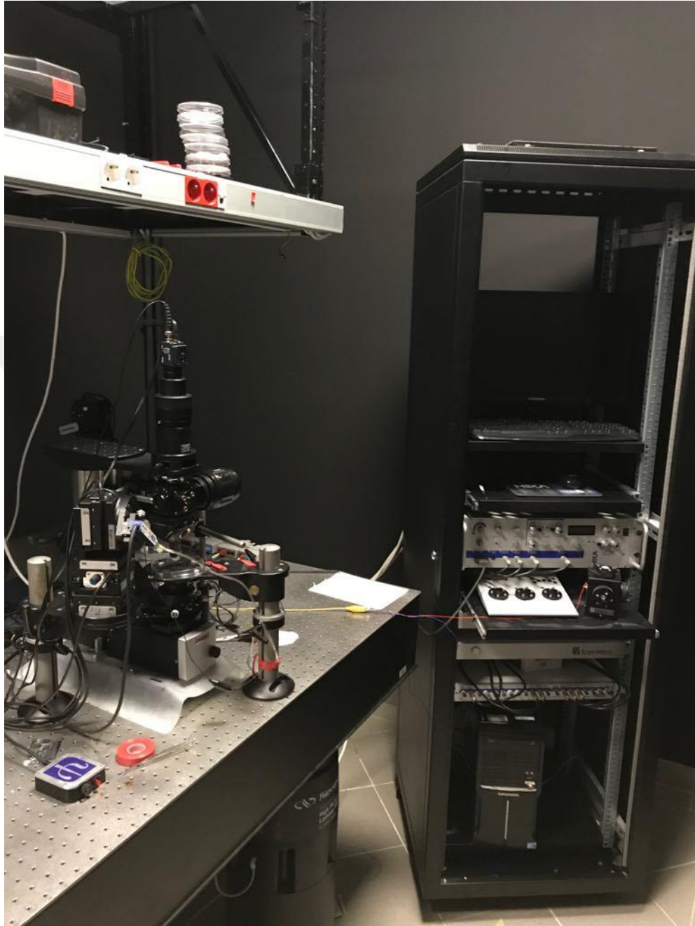
Figure 24: Patch clamp setup in our lab. On the right, computer, patch clamp amplifier and microcontrollers for microscope and pipette holder can be seen. On the left, microscope, pipette holder, optical setup and sample holder is located on the optical table.
