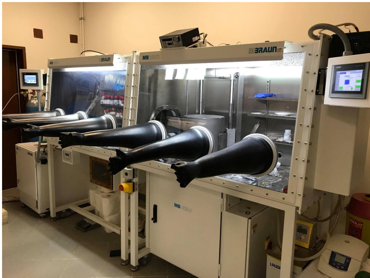
Figure 9: Nitrogen glove box in our laboratory, where the most part of the QLED fabrication takes place.
