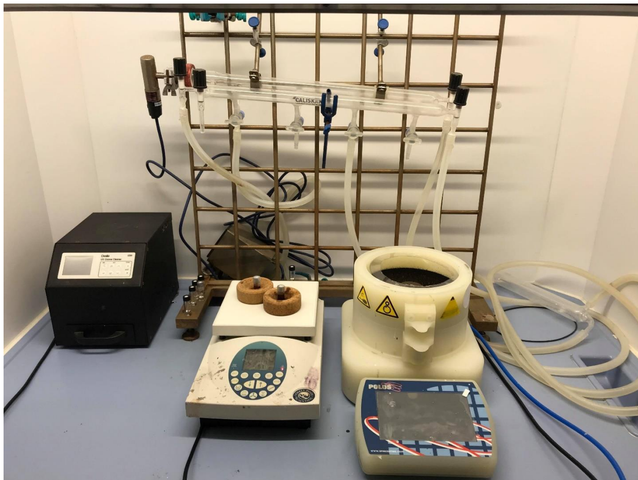
Figure 21: Photoelectrode fabrication instruments. From left to right: UV ozone cleaner, high sensitivity heater, and spin coater.
