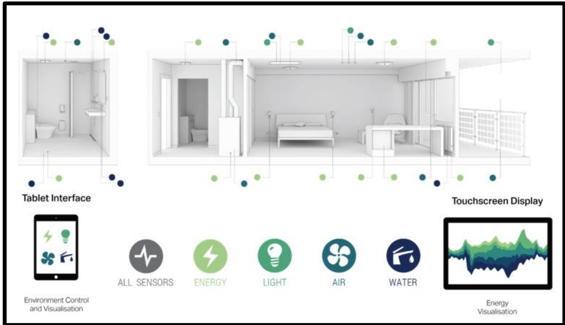
Figure 3.20: Shows the Smart Aspect of the Green Solution House With the Intelligent Control Through Tablet and Touch Screen Display to Control Rooms Energy, Light, Air, and Water for Best Experience and Efficiency (GXN, 2015).
