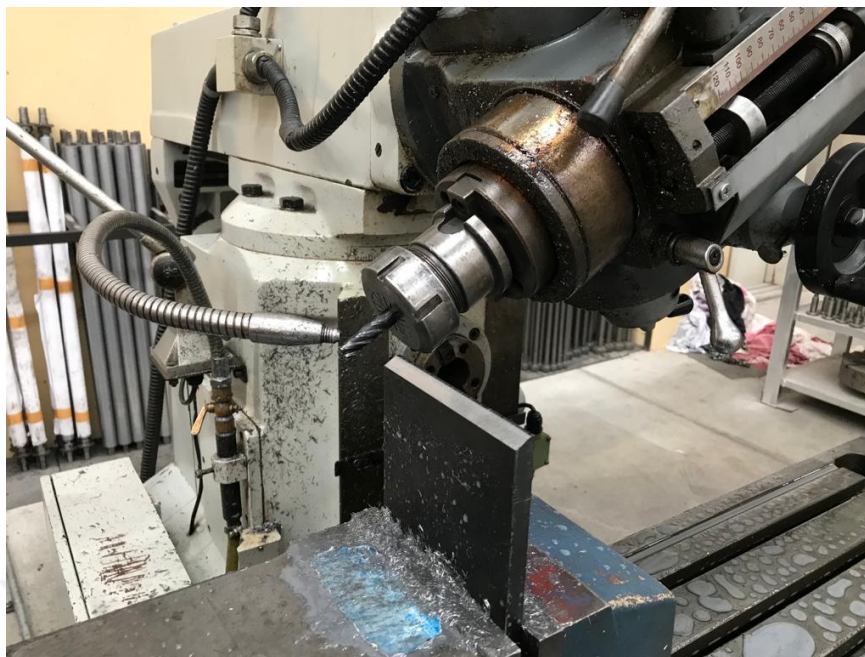
Figure 3.3 The machined material to obtain groove angle of 60^\circ and root face of 2 mm
