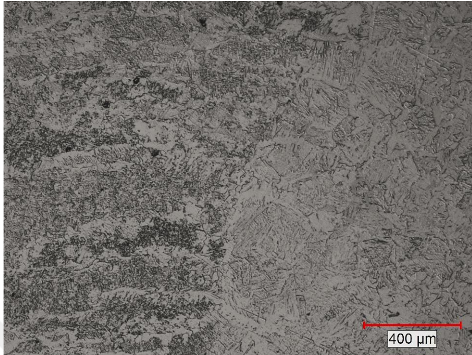
Figure 4.27 Transition zone from the HAZ region to the weld metal (Sample B); 50x
