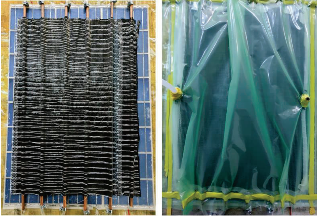
Figure 2.27 Preparation of the cooling system components for VARTM-based production.
