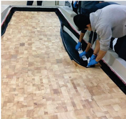
(b) Placement of core materials
