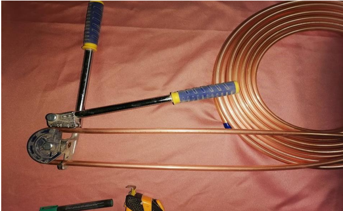
Figure 3.9: Bending Process of the Copper Tube.
