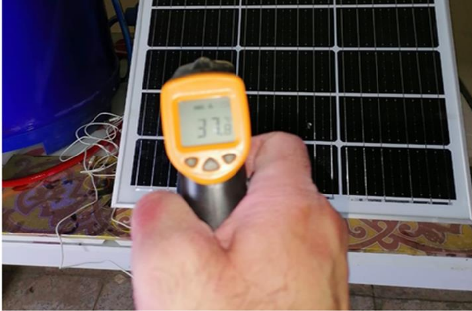
Figure 3.12: Panel Surface Temperature Measurement.
