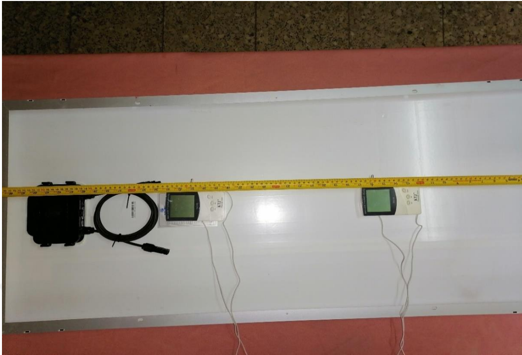
Figure 3.11: Thermal Sensor Position at the PV Panel.
