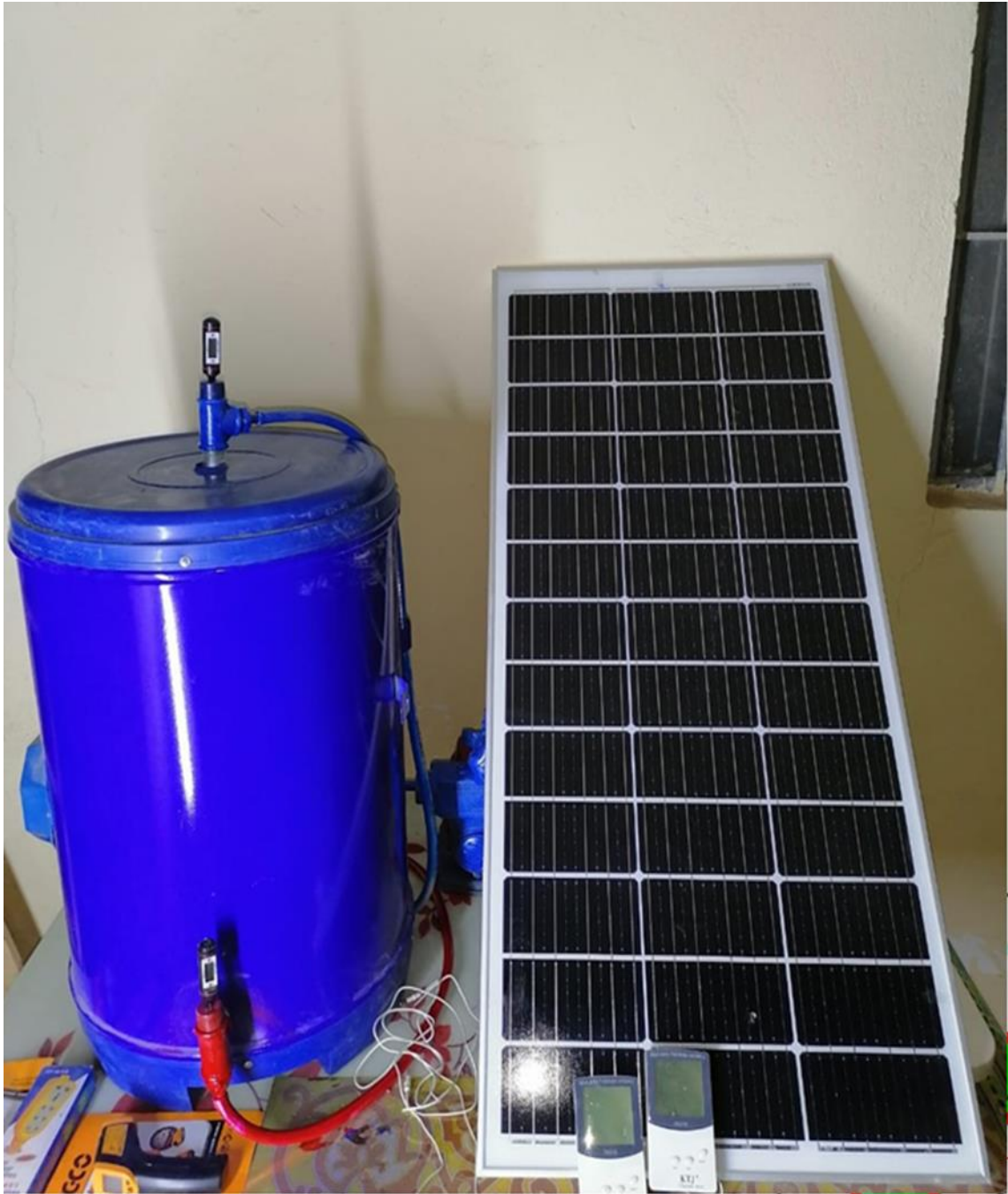
Figure 3.3: Experimental Prototype of all System: PVT Collector.
