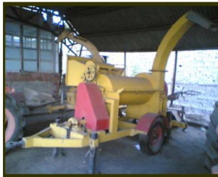
Figure 3.8: Dry Feed Shredder Takes Power from Tractor Back Shaf
