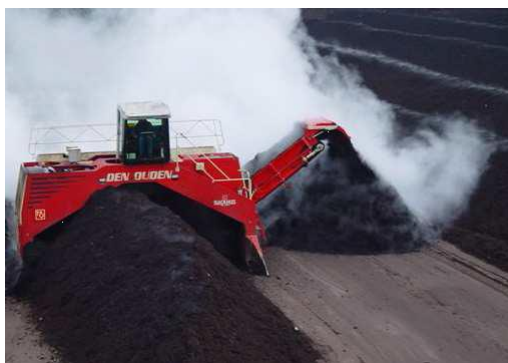
Figure 3.11: Self-Propelled Compost Stirrers for the Adjacent Site
