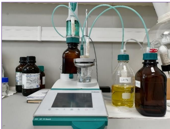
Figure 3.19: Automatic titration instrument used for Volumetric KF Titration.
