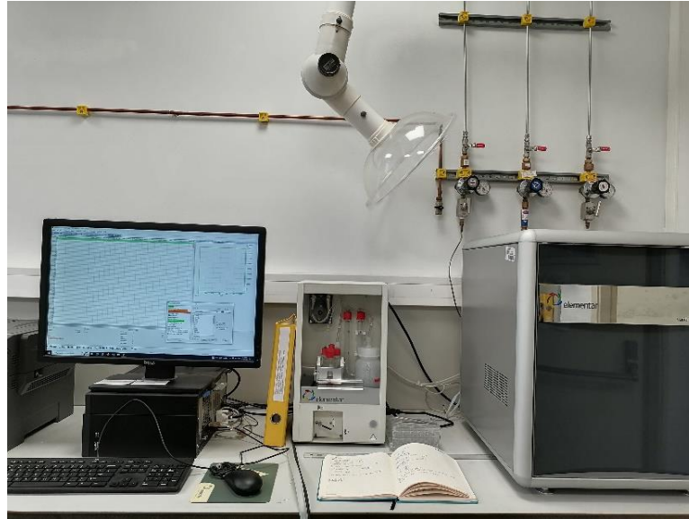
Figure 3.7: The elemental analyzer used in the ultimate analysis of composite wastes.
