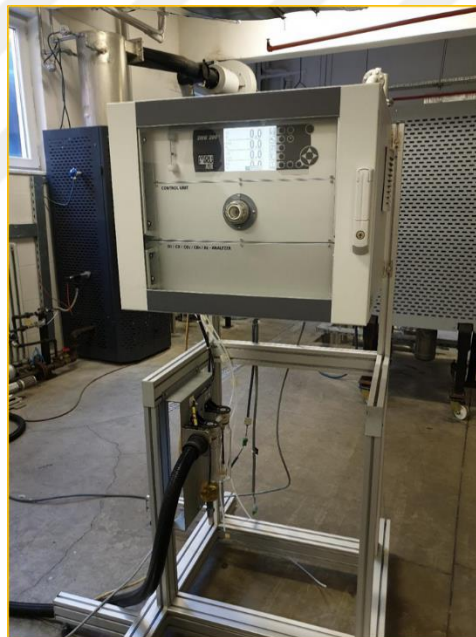
Figure 3.12: Online syngas analyzer used in pyrolysis test.
