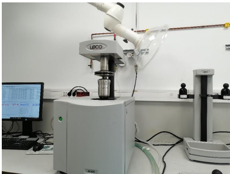
Figure 3.8: Automatic calorimeter used to determine samples' calorific values.
