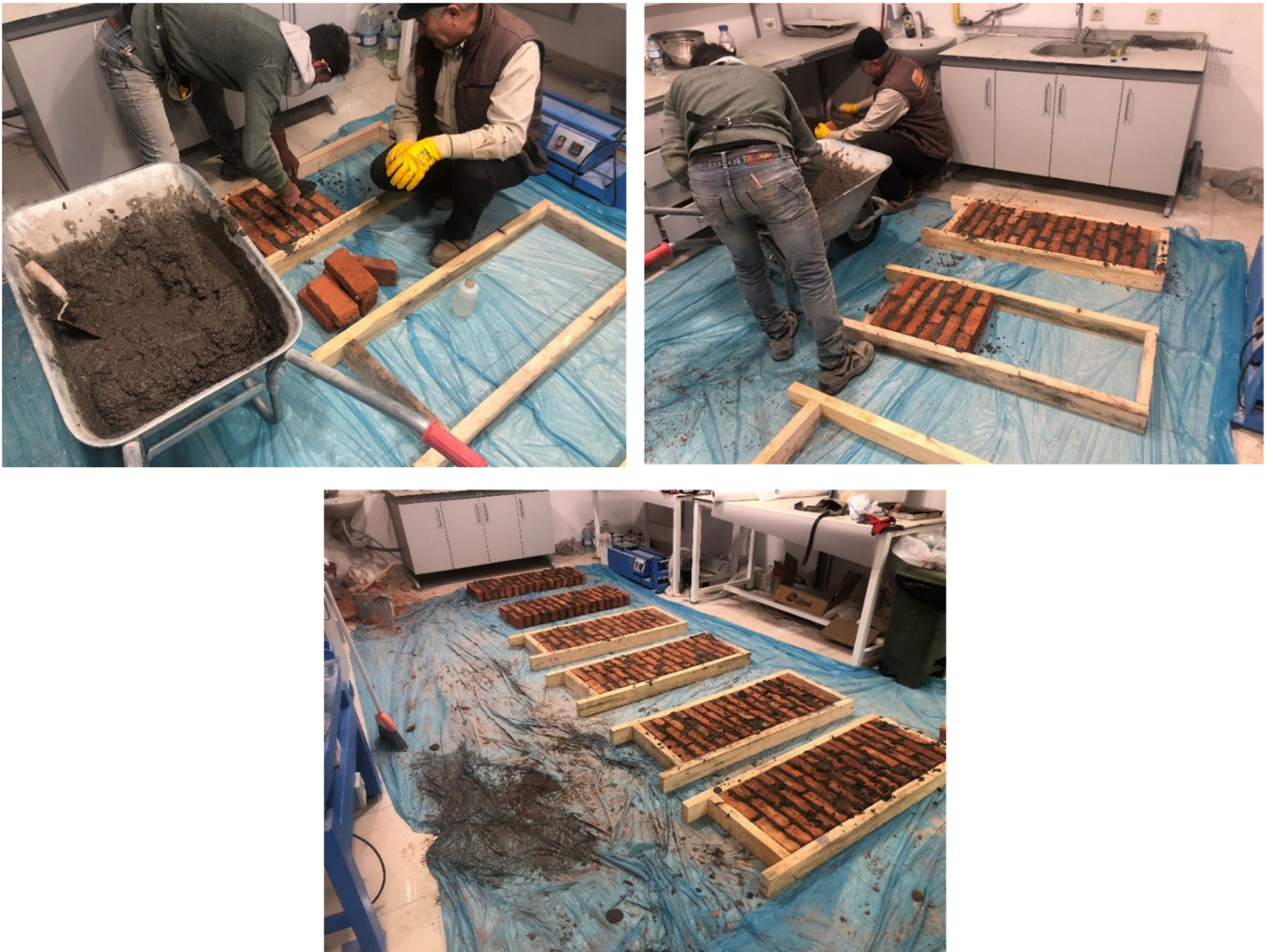
Figure 3.3 Production processes of masonry panels
