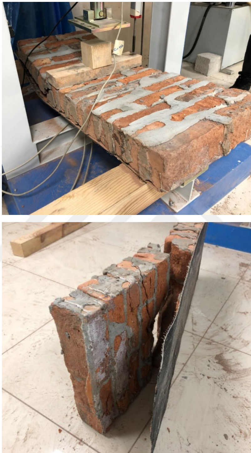
Figure 4.18 Testing & Failure mode of S-F-L2
