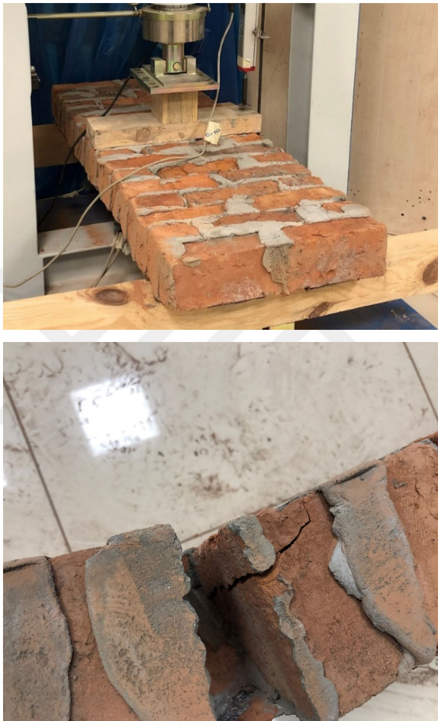
Figure 4.12 Testing & Failure mode of S-S2-L2
