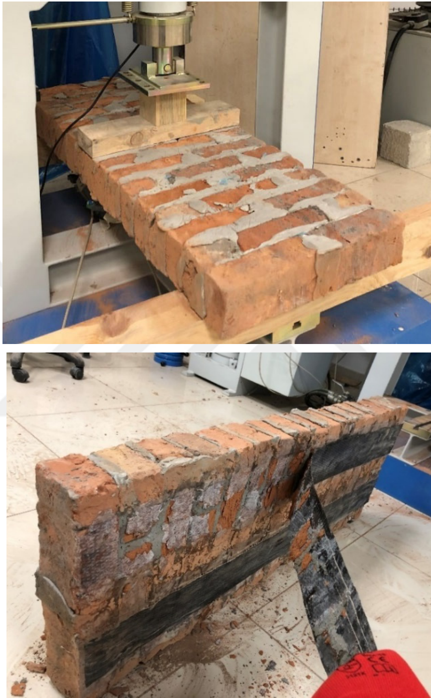
Figure 4.10 Testing & Failure mode of S-S2-L1
