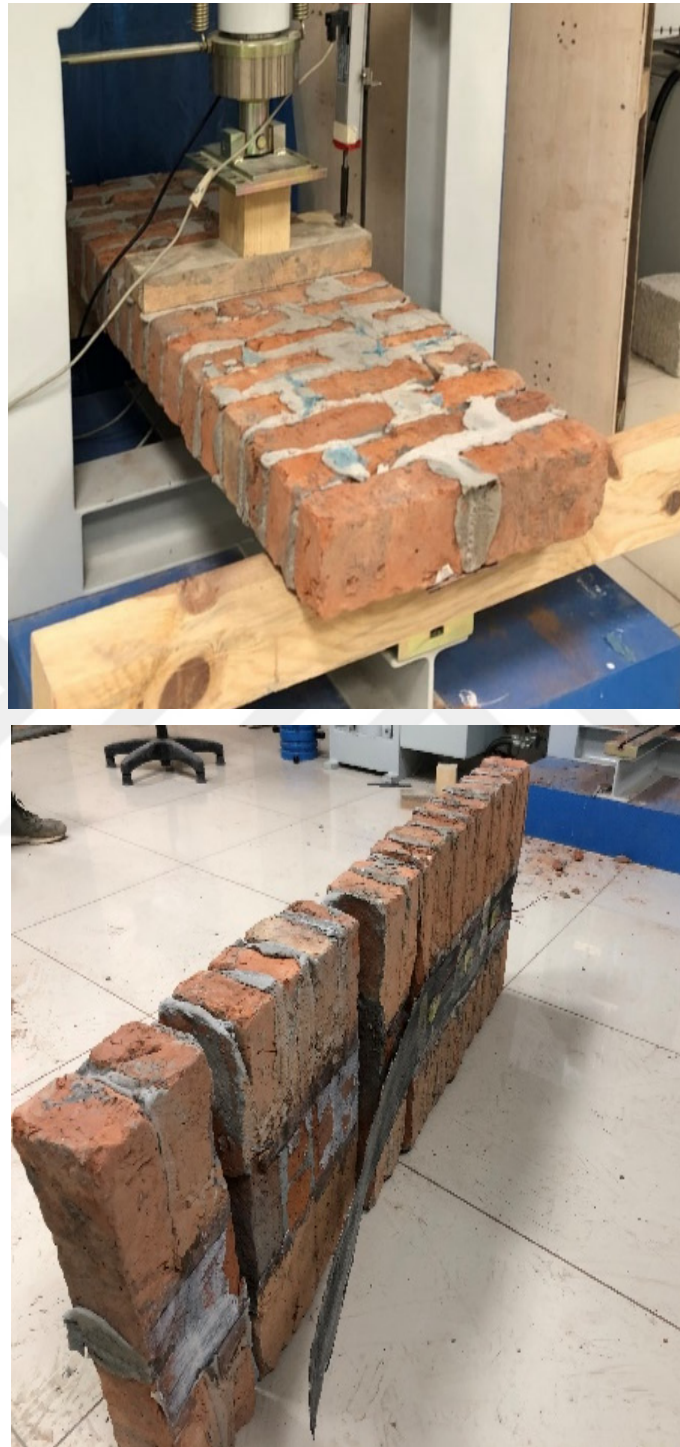
Figure 4.4 Testing & Failure mode of S-S1-L1
