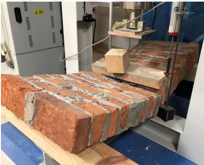
Figure 4.2 Testing & Failure mode of control specimen
