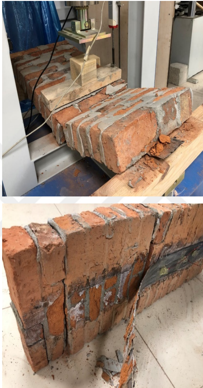
Figure 4.6 S-S1-L2 Testing & Failure mode.
