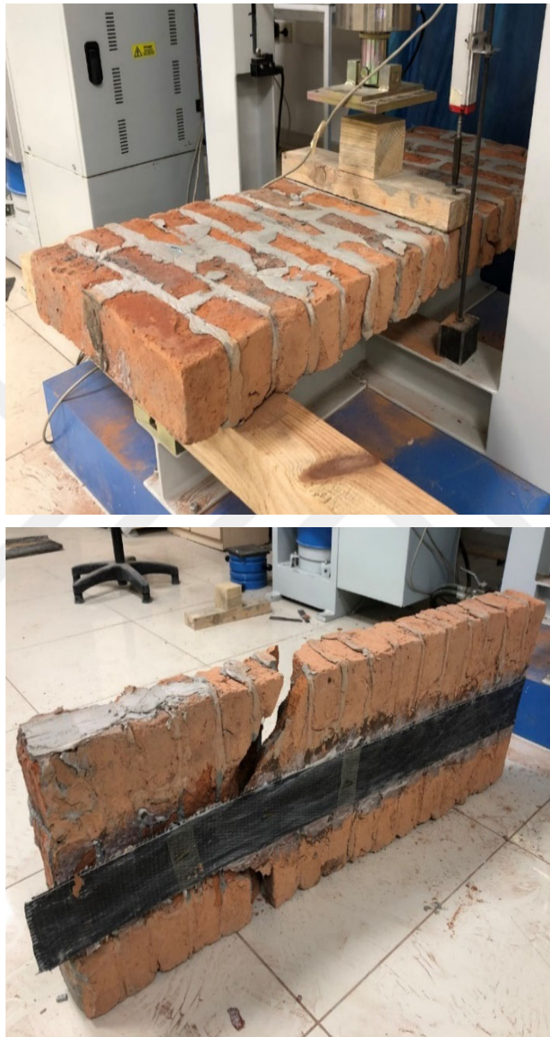
Figure 4.8 Testing & Failure mode of S-S1-L3
