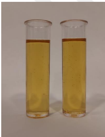
Figure 3. 9 Untreated and treated used frying oil samples with MgSi at 180 °C (from left to right)
