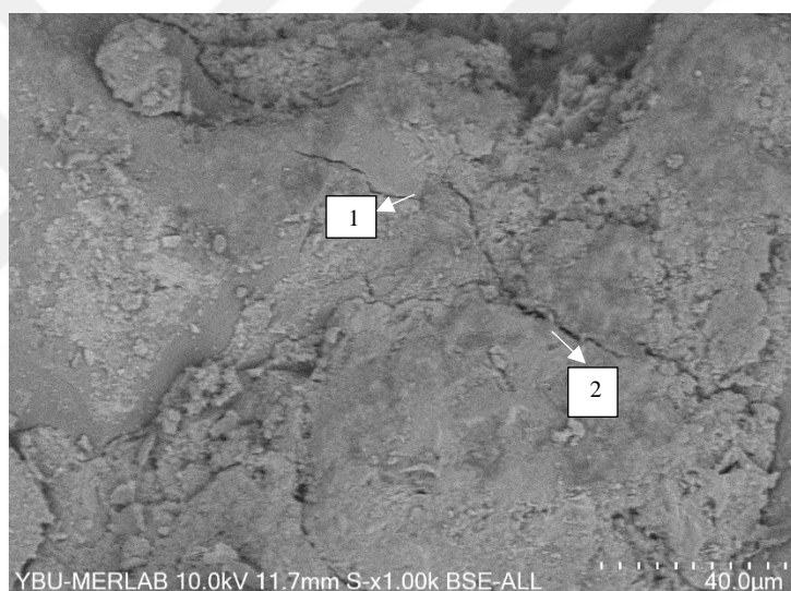
Figure 4.34 Cracks that appeared on the surface of mortar paste.
