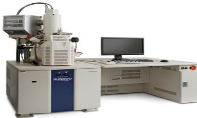
Figure 3.11 Scanning electron microscopy device with Energy Dispersive X-Ray Spectroscopy (SEM/EDX).
