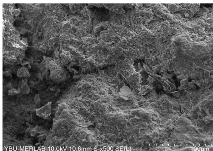
Figure 4.30 SEM image of aggregate (A) at w/c: 0.4 with curing temperature of 60°C.
