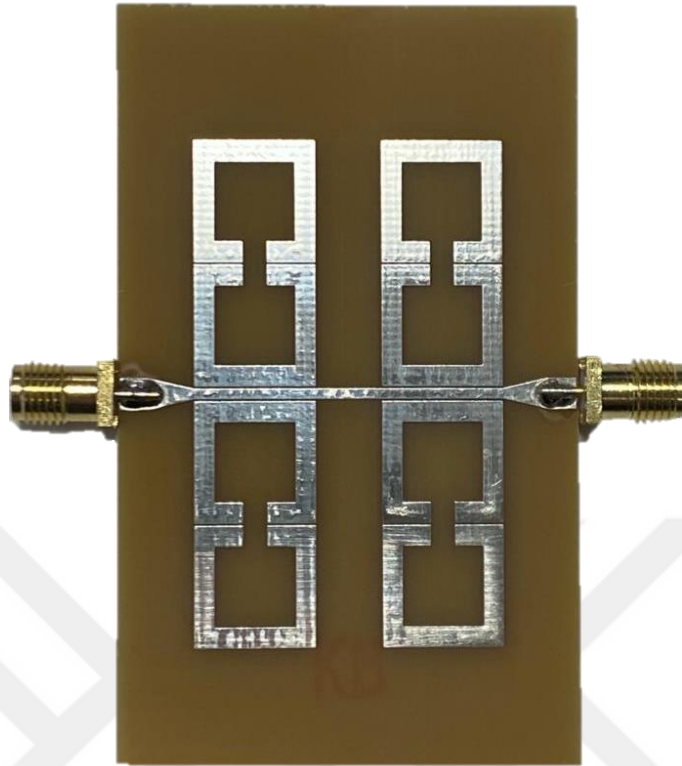
Figure 4.1. Manufactured FR-4 Filter
