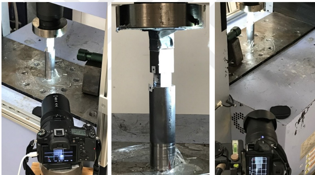
Figure 2.22. Out-of-plane off-axis compression test system (a) camera-1, (b) specimen, and (c) camera-2
