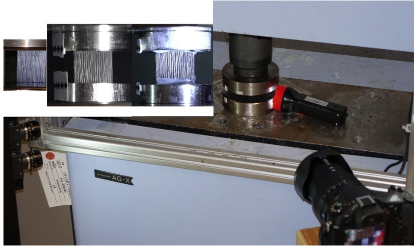
Figure 2.12. Quasi-static compression tests on cubic samples
