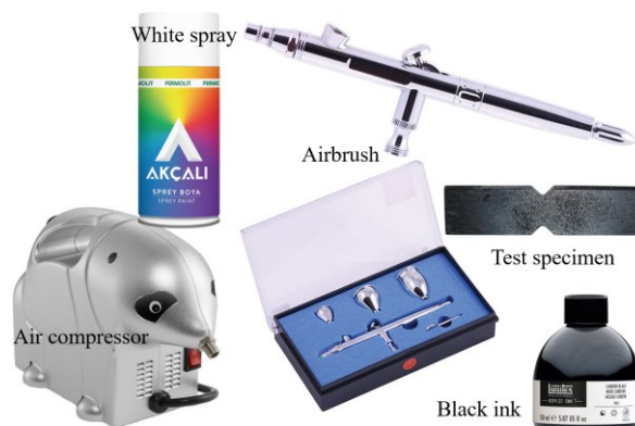
Figure 2.4. Equipment used in specimen preparation for DIC
