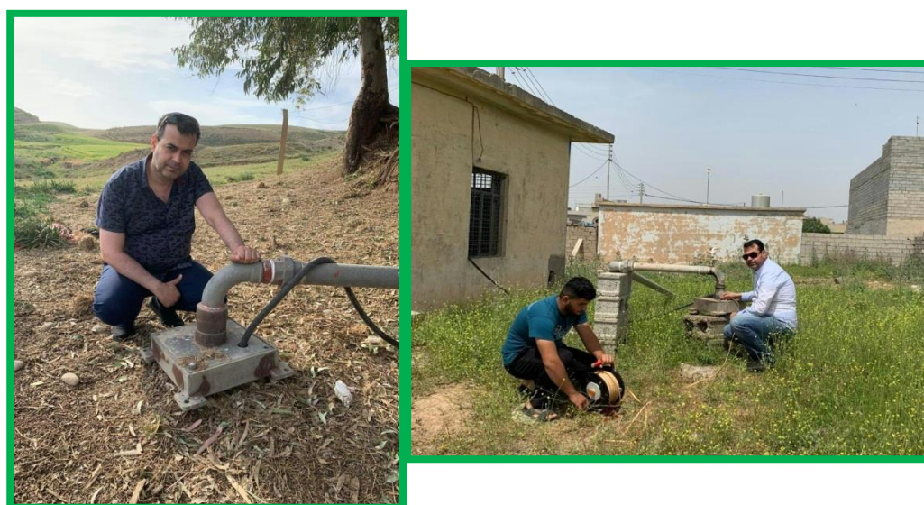
Figure 2.2. Static water level measuring for the wells in the study area using a water level meter
