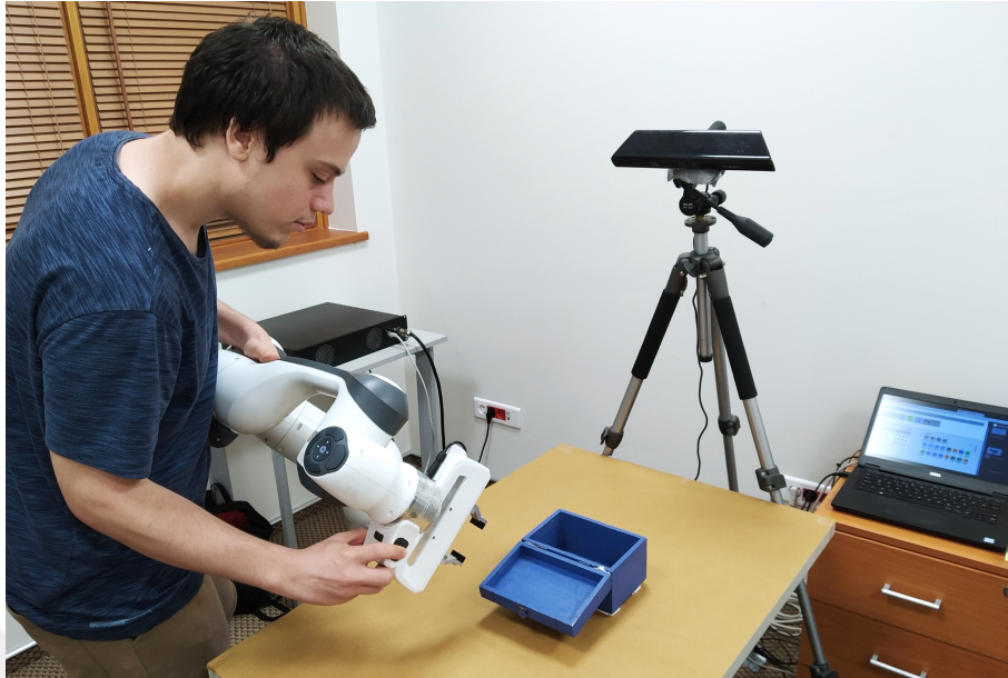
Figure 3.1: Demonstration. The picture depicts a user providing close box skill demonstration with a robotic hand (Pand robot by Franka Emika). The robotic hand in white, an object of interest on top of the table in blue and a RGB-D scanner (Microsoft Kinect) on a stand to capture perceptual data.
