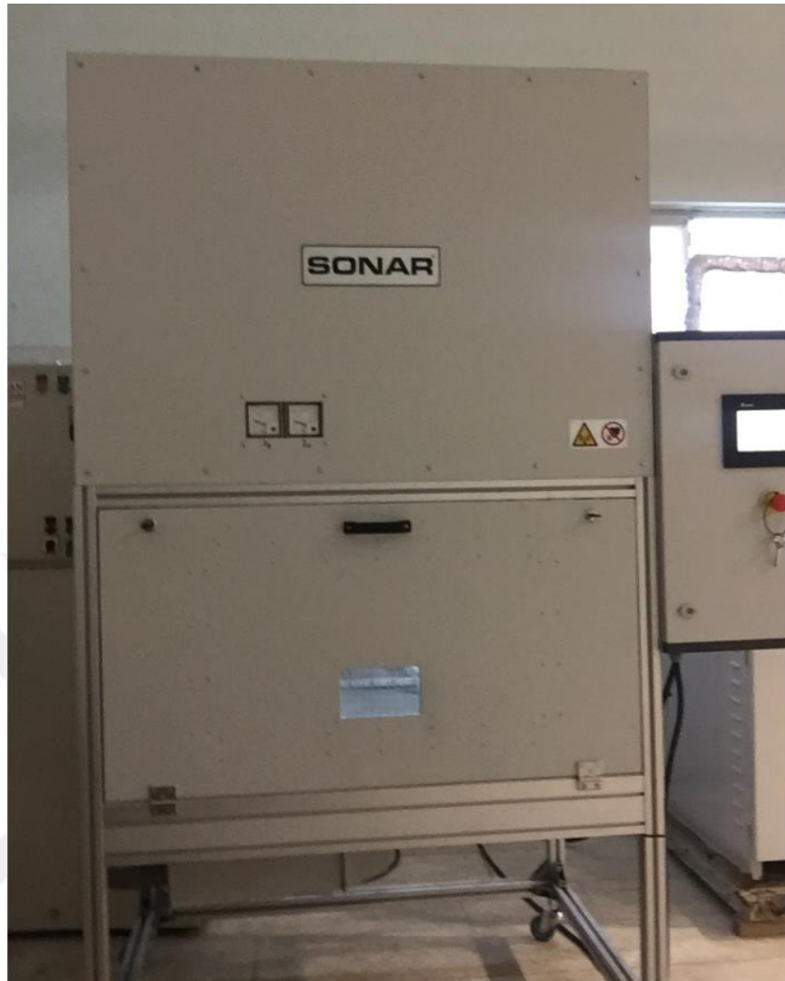
Figure 3.1 Hot Air Assisted RF Drying System
