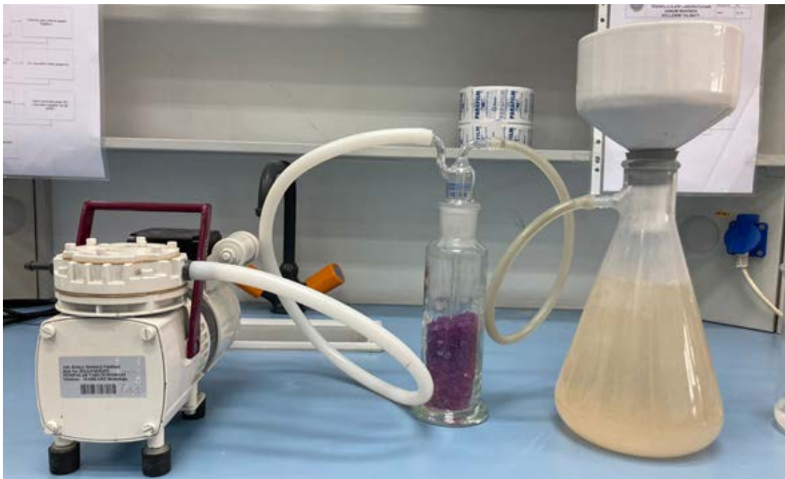
Figure 6.8 Filtration after deproteinization of crab shells
