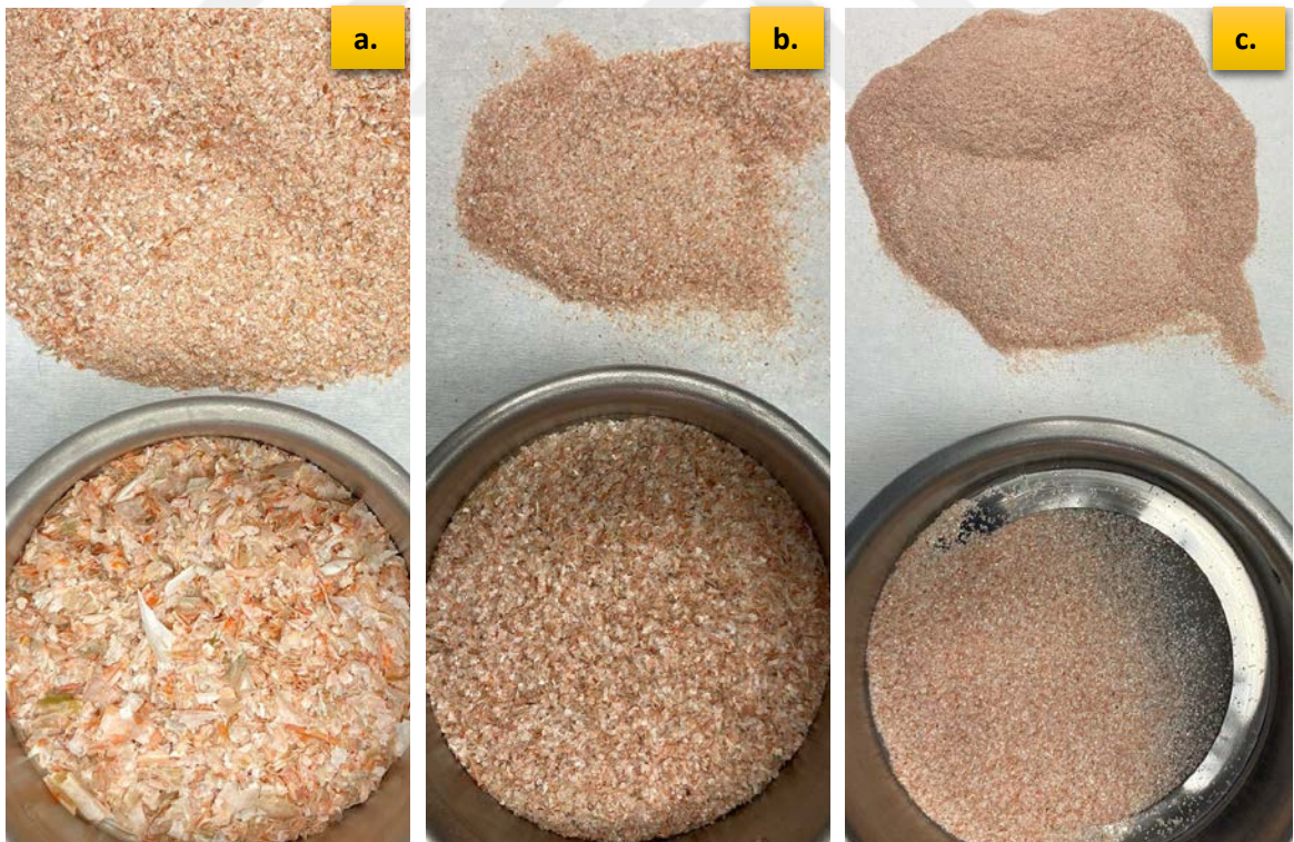
Figure 6.5 Shrimp shells divided into sieve meshes a. -40, +18 mesh, b. -60, +40 mesh, c. +60 mesh
