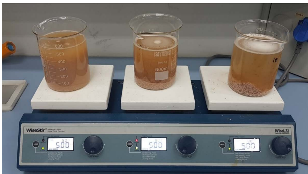
Figure 6.6 Deproteinization of crab shells
