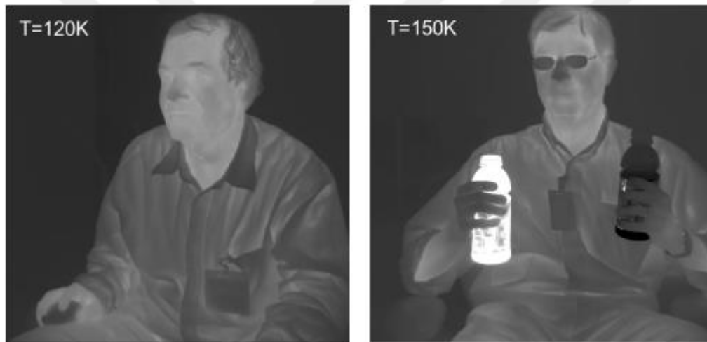
Figure 2.22: The images taken with 2k \times 2k superlattice-based FPA at 120 K and 150 K, respectively [91].
