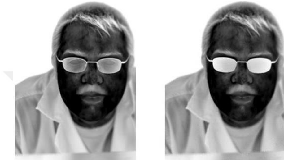
Figure 2.15: Thermal images taken with dual-color FPA. The left is the blue channel, and the right is the red channel [83]. White regions correspond to the colder places.
