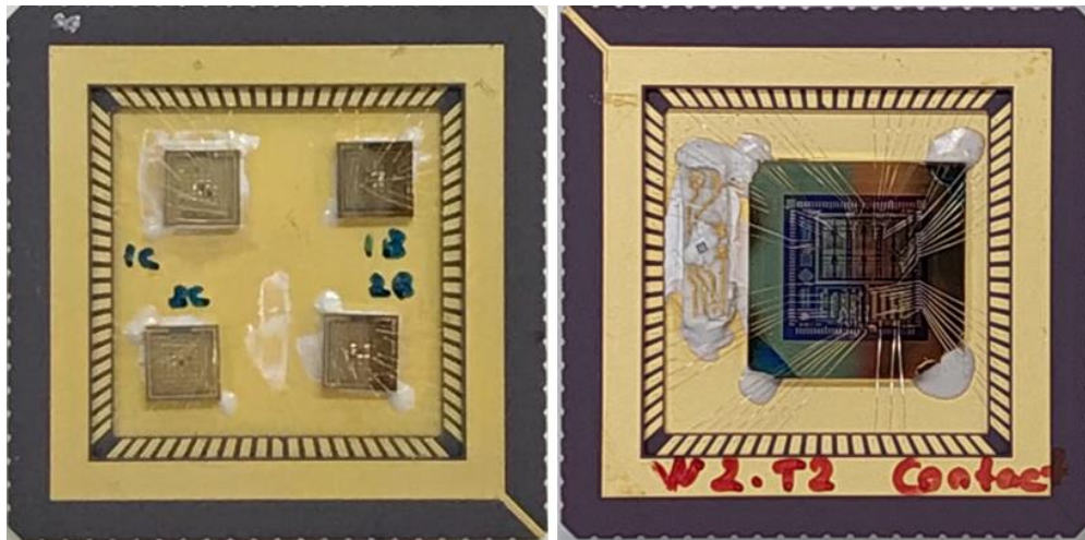
Figure 3.37: The packaged MAPO samples (left) and SLS-TEST sample (right) for measurements.
