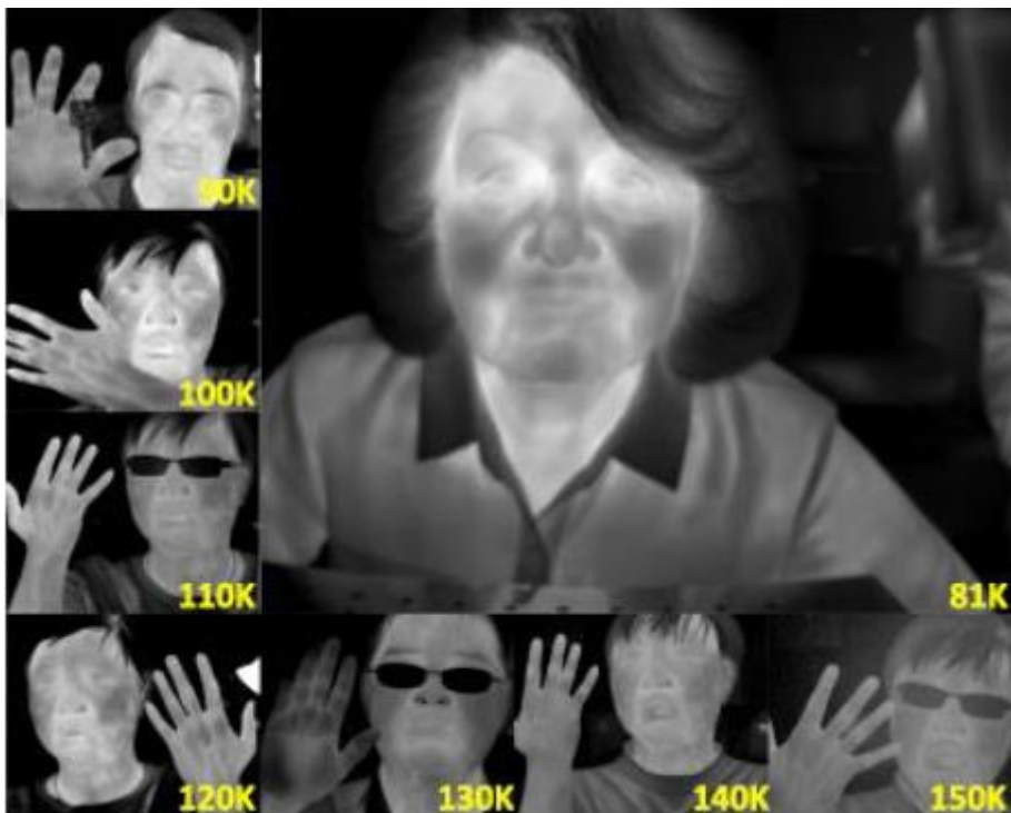
Figure 2.19: Thermal images taken with 320 \times 256 pixel format FPA at temperatures from 81 K to 150 K [87].
