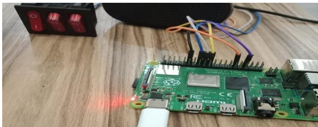
Figure 22 Switch buttons connection with the RPi
