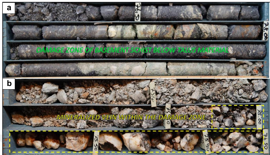
Figure 4.9. Damage zone at the transition between talus and the basement graphitic schist unit in Sırakayalar, a) highly-deformed and locally clay-rich graphite-mica schist in drill hole SHD-236 (76.00 – 80.00 m), b) mineralized vein emplaced within highly-deformed graphite -mica schist in drill hole SHD-249A (73.00 – 76.50 m).
