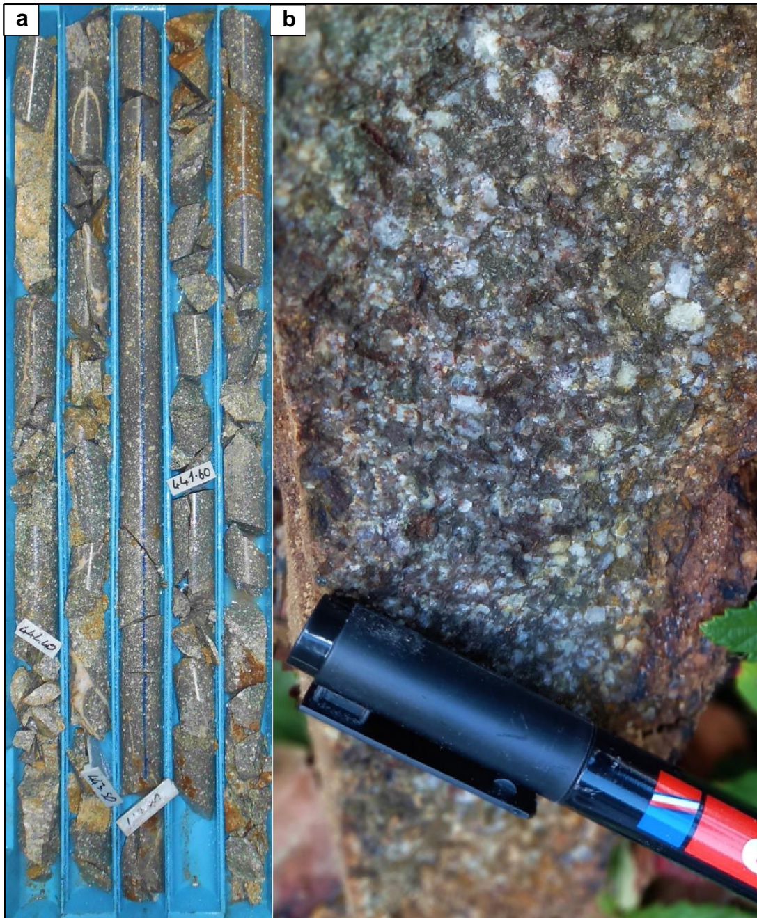
Figure 4.4. Least-altered samples of porphyritic unit in Karatepe Sector comprises large phenocrysts of plagioclase, amphibole, and minor K-feldspar and quartz set in a fine-grained groundmass of plagioclase and quartz. a) 440.20 to 444.60 m interval of dacite from SHD-107A drillhole, b) hand sample of least-altered dacite porphyry from the Karatepe Sector (481963E, 4463053N, 295 meters a.s.l.).
