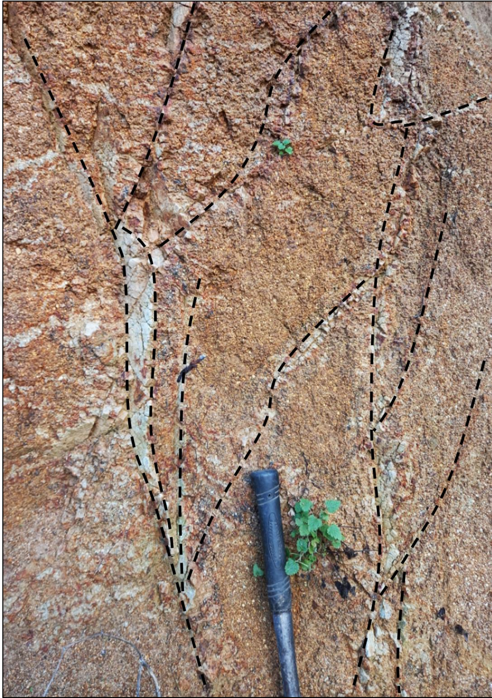
Figure 4.12. Sheared and altered dacite porphyry in Karatepe Zone (481971E, 4463049N, 294 m elevation; UTM Zone 35S).
