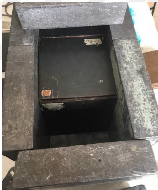
Figure 28. The Graded Shielding Geometry with Iron
