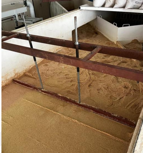
Figure 3.20: The apparatus to obtain a horizontal bed along the main channel
