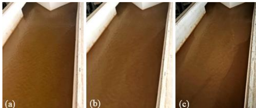
Figure 4.10: The view of bed morphology for E2 (a) 3 h, (b) 9 h, (c) 15 h
