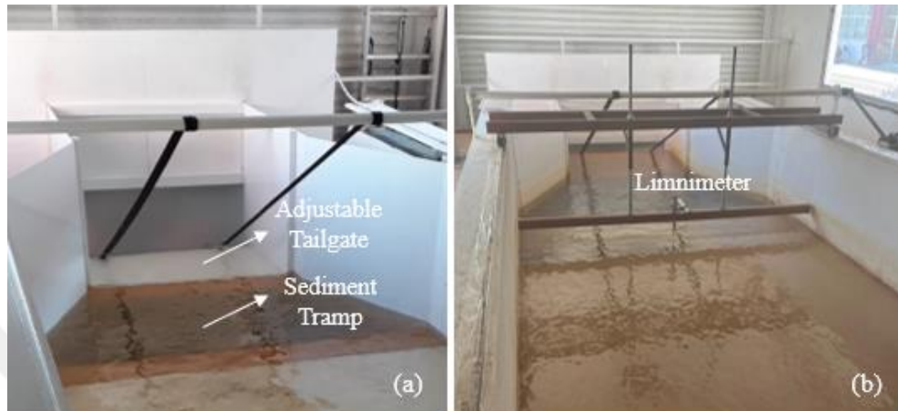
Figure 3.11: (a) Adjustable tailgate, (b) Limnimeter
