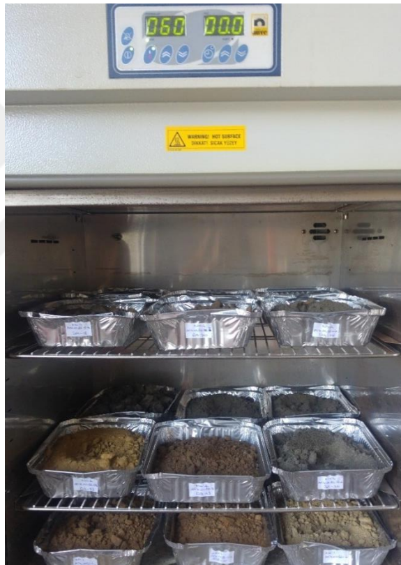
Figure 3.8 Dried the waste samples at 60 °C
