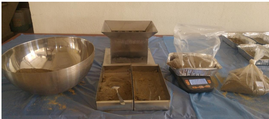
Figure 3.9 The use of a riffle splitter for homogenous mixing
