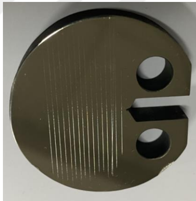
Figure 22. Fatigue crack growth sample and drawn lines
