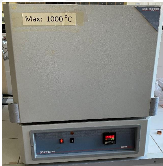
Figure 8. Aging heat treatment furnace
