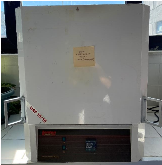
Figure 7. Solution heat treatment furnace
