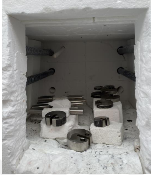
Figure 9. All samples in the furnace for solution heat treatment and aging
