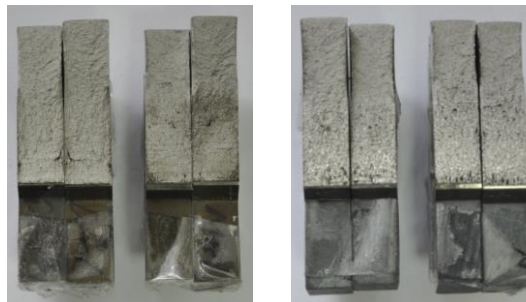
Figure 88. Fracture surface of 200 and 200H
