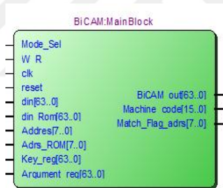
Figure 5.7 : Block diagram Symbol of the proposed FPGA-based BiCAM.
