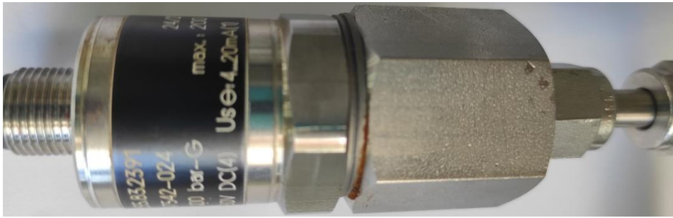
Figure 4.5 Leak through pressure sensor and PMRS connection occurred during with the Al6061-07 tube storage
